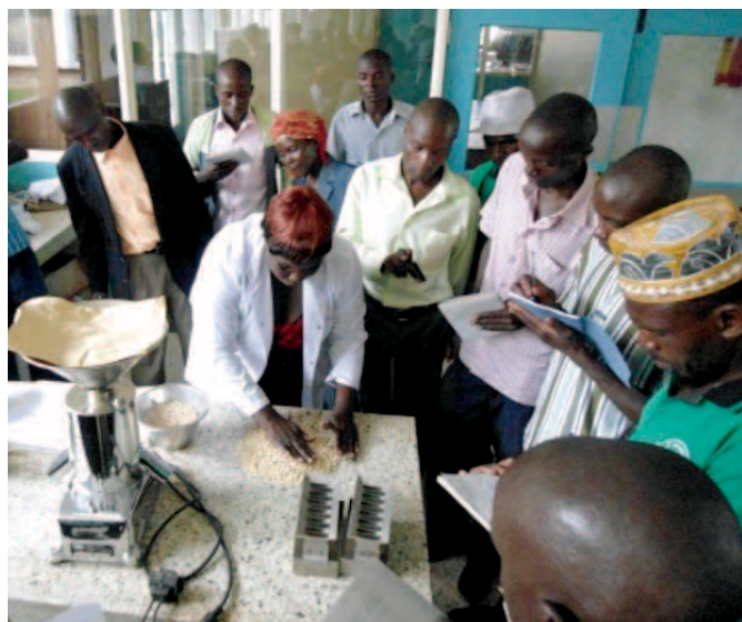
A seed analyst explains how to obtain a working sample for seed testing
